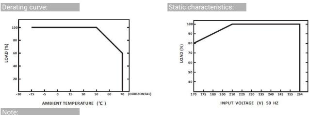
The given parameters (unless otherwise stated) were measured for a supply voltage of 230V AC, at nominal load in laboratory conditions, at an ambient temperature of 25°C.
